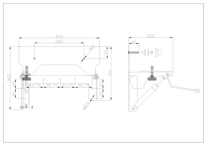
Pneumatic tilting bracket mechanism for washbasin, made of painted steel
