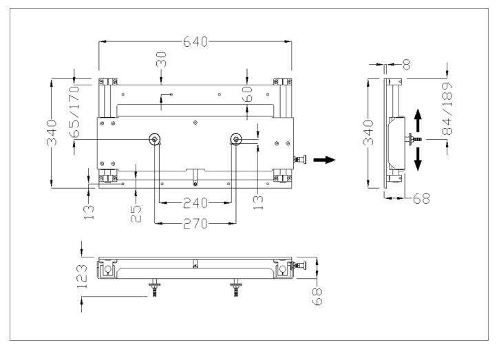
Pneumatic wash basin high-low device, made of painted steel
