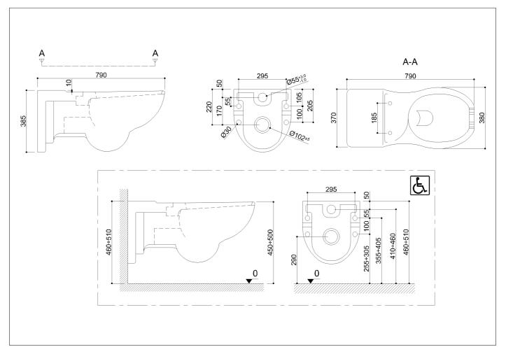
Open front wall-hung WC pan made of vitreous china
