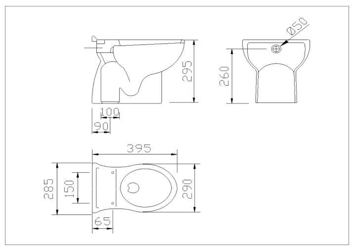
WC pan made of vitreous china with decoration in relief. Floor drain
