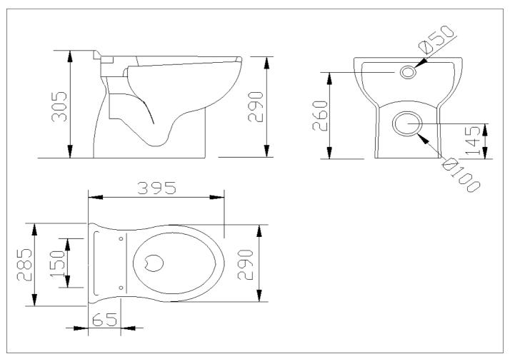
WC pan made of vitreous china with decoration in relief. Wall drain
