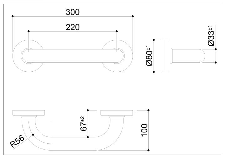
Straight grab bar made of seamless zinc-plated steel pipe, coated with biocompatible and warm-to-the-touch vinyl
