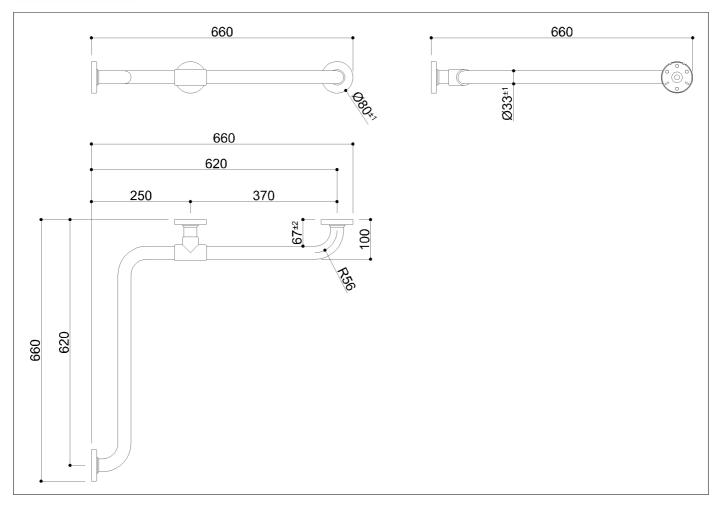
Corner grab bar made of zinc-plated steel pipe, coated with biocompatible and warm-to-the-touch vinyl
