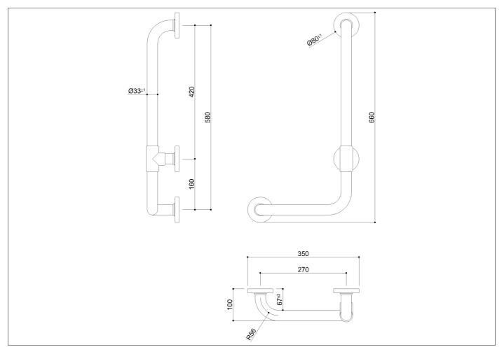
L-shaped grab bar made of zinc-plated steel pipe, coated with biocompatible and warm-to-the-touch vinyl
