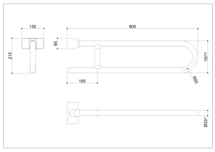
Folding grab bar with reinforced joint made of seamless zinc-plated steel pipe, coated with biocompatible and warm-to-the-touch vinyl
