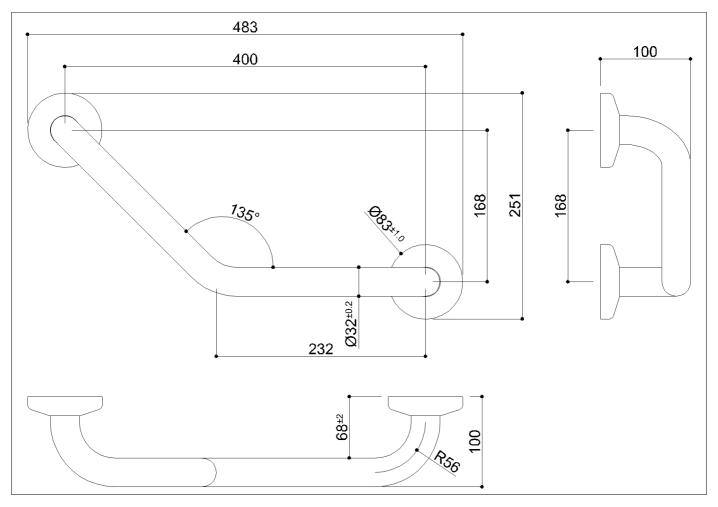
135° angled grab bar made of seamless steel pipe, painted with synthetic thermoplastic powder of plant origin, Rilsan®
