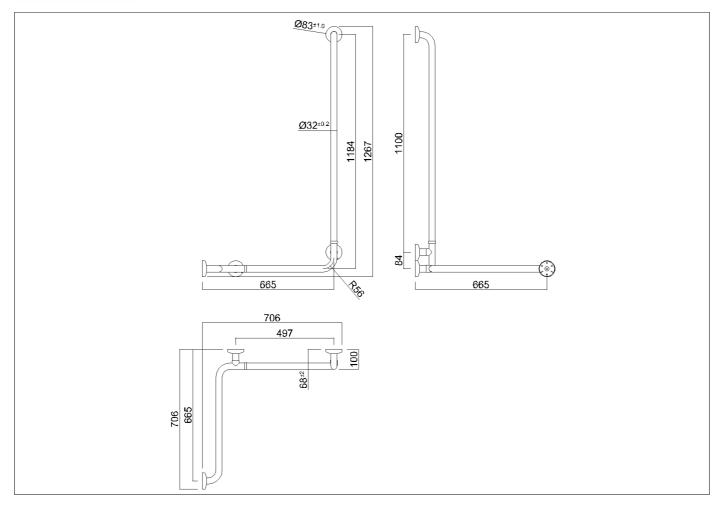
Vertical and horizontal safety support made of seamless steel pipe, painted with synthetic thermoplastic powder of plant origin, Rilsan®  $\,$
