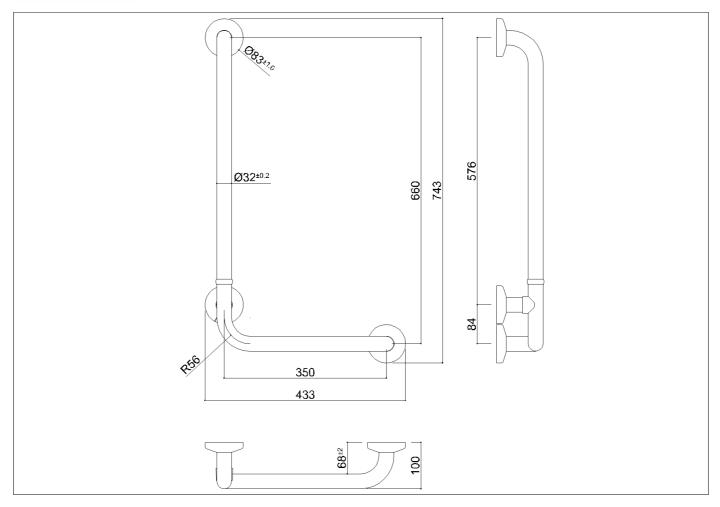
L-shaped support made of seamless steel pipe, painted with synthetic thermoplastic powder of plant origin, Rilsan®
