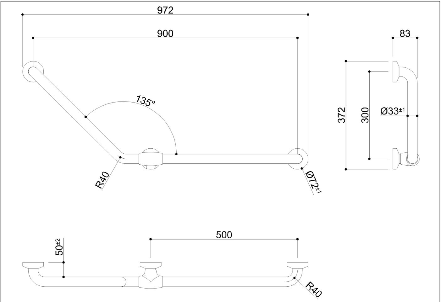
Safety corner grab rail 135° Ø 33 mm with antislip, vinyl coating and zinc-plated steel internal pipe without junctions. Active and long lasting antimicrobial protection based on silver ions. Wall clearance 50 mm. Concealed wall fixing kit Ø 72 mm, in stainless steel with base plate, for wall protection, and external cover made of polyamide-6.
