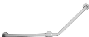
Safety corner grab rail 135° Ø 33 mm with antislip, vinyl coating and zinc-plated steel internal pipe without junctions. Active and long lasting antimicrobial protection based on silver ions. Wall clearance 50 mm. Concealed wall fixing kit Ø 72 mm, in stainless steel with base plate, for wall protection, and external cover made of polyamide-6.
