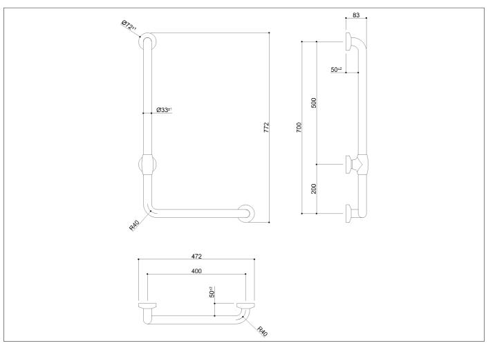
Safety corner grab bar  $90^{\circ}$  Ø 33mm with antislip, vinyl coating and zinc-plated steel internal pipe without junctions. Active and long lasting antimicrobial
