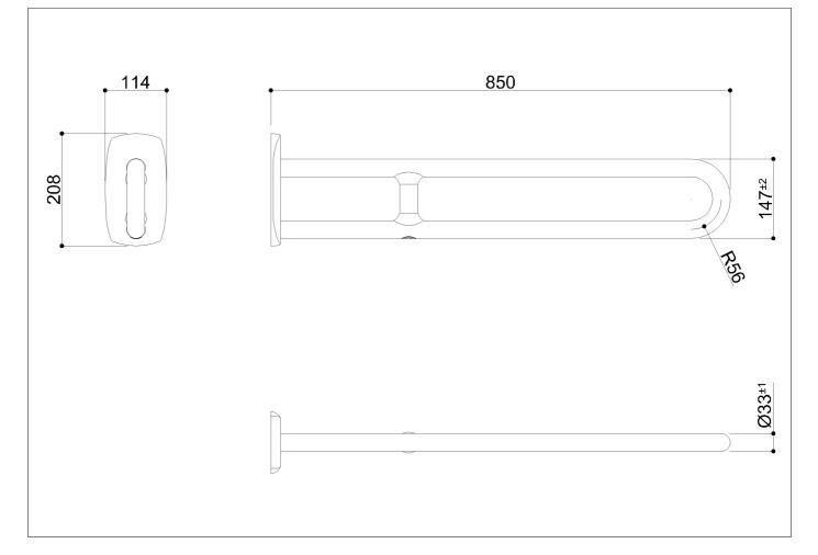
Side fixed safety support. Wall fixing kit in stainless steel with Polyamide-6 cover. Base plate in polyamide for wall protection. Grab rail Ø 33mm with vinyl coating and zinc-plated steel internal tube. Active and longlasting antimicrobial protection based on silver ions.
