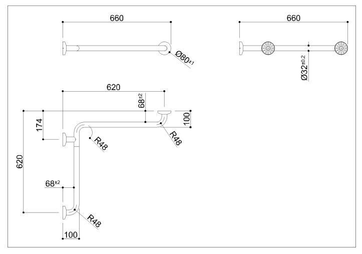
Polished stainless steel safety handrail, Ø 32x1.5 mm in AISI 304 stainless steel, no junctions. Wall clearance 50 mm. Concealed wall fixing kit Ø 80 mm with stainless steel flange cover and flange. Fit for installation in bath and toilet areas, to enable the person to grab for elevating from lower position. Left or right assembling.
