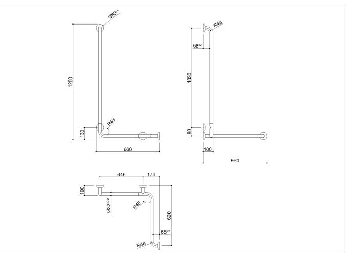
Polished stainless steel safety handrail for corner installation with vertical arm  $\emptyset$  32x1.5 mm in AISI 304 stainless steel, no junctions.
