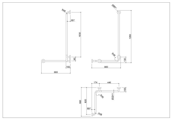
Polished stainless steel safety handrail for corner installation with vertical arm Ø 32x1.5 mm in AISI 304 stainless steel, no junctions. Wall clearance 50 mm.
