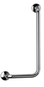
Polished stainless steel safety corner grab rail, Ø 32x1.5 mm in AISI 304 stainless steel, no junctions. Wall clearance 50 mm. Concealed wall fixing kit Ø 80 mm with stainless steel flange cover and flange. Fit for
