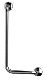
Polished stainless steel safety corner grab rail, Ø 32x1.5 mm in AISI 304 stainless steel, no junctions. Wall clearance 50 mm. Concealed wall fixing kit Ø 80 mm with stainless steel flange cover and flange. Fit for
