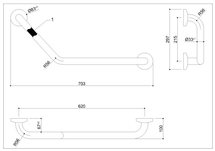
135° angled grab bar made of seamless zinc-plated steel pipe, coated with antimicrobial, biocompatible and warm-to-the-touch vinyl
