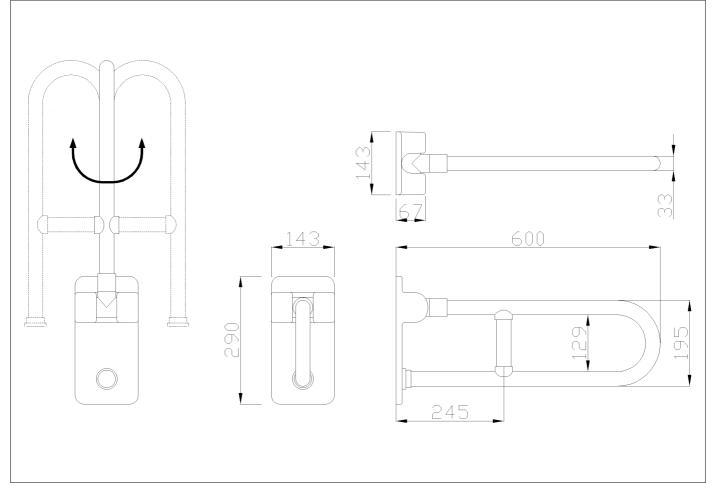
Folding and rotating grab bar with reinforced joint made of seamless zincplated steel pipe, coated with antimicrobial, biocompatible and warm-to-thetouch vinyl
