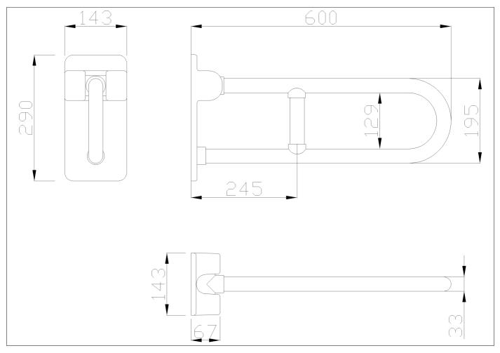
Folding grab bar with reinforced joint made of seamless zinc-plated steel pipe, coated with antimicrobial, biocompatible and warm-to-the-touch vinyl
