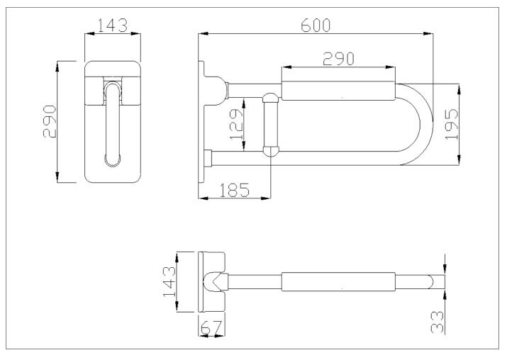
Folding grab bar with reinforced joint made of seamless zinc-plated steel pipe, coated with antimicrobial, biocompatible and warm-to-the-touch vinyl. Equipped with soft armrest
