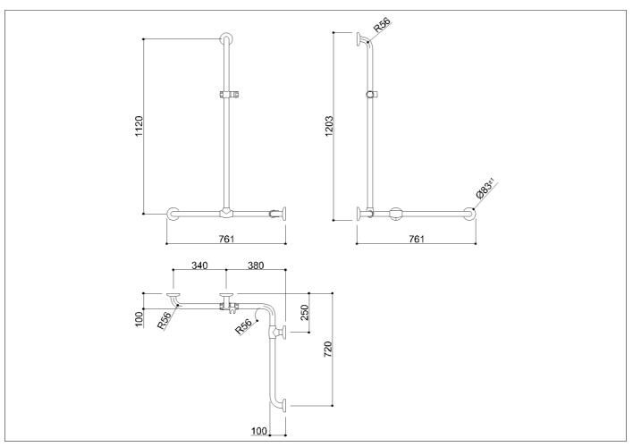
Corner and vertical grab bar made of zinc-plated steel pipe, coated with antimicrobial, biocompatible and warm-to-the-touch vinyl. Equipped with hand shower holder
