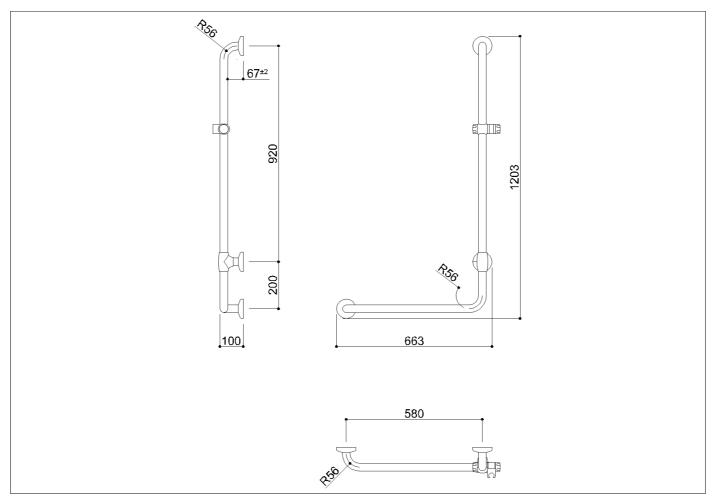
L-shaped grab bar made of zinc-plated steel pipe, coated with antimicrobial, biocompatible and warm-to-the-touch vinyl. Equipped with hand shower holder
