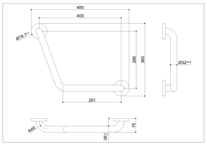
110° angled grab bar made of seamless stainless steel AISI 304 pipe, with satin finish
