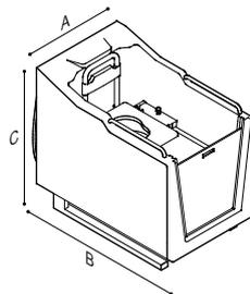
**800\_SHOWER CUBICLE, EQUIPPED WITH BACKREST AND SUPPORT HANDLES MADE OF STAINLESS STEEL WITH SATIN FINISH**
