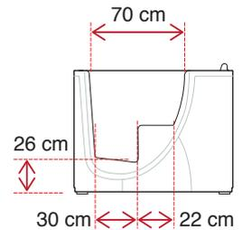
The width of the door makes a sufficient portion of the seat accessible, so it is possible to enter the bathtub either standing or sitting, making it the only one of its kind.
