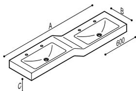
**MILK\_ FOUR-PLACE CONSOLE SINK ON DOUBLE HEIGHT TOP, EQUIPPED WITH BRACKETS**
