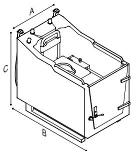
**700\_WATERTIGHT BATHTUB, WITH BUILT-IN CONTROL PANEL, EQUIPPED WITH BACKREST AND SUPPORT HANDLES MADE OF STAINLESS STEEL WITH SATIN FINISH**
