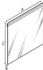
**HUG FIXED MIRROR, 5 MM THICK, WITH BUILT-IN LED LIGHTING SYSTEM AND SWITCH, WITH TOUCH SENSOR**
