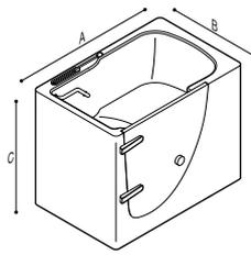
**651\_ BATHTUB WITH DOOR WITH OUTWARD OPENING, EQUIPPED WITH GRAB BAR ON BATHTUB BODY**
