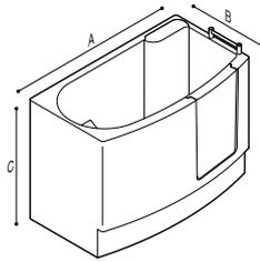
**653\_ BATHTUB WITH DOOR, INWARD OPENING, EQUIPPED WITH SUPPORT GRAB BAR**
