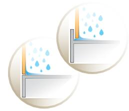
A traditional shower base requires sealing between the base and the coating. The solution with base equipped with lateral containment profile - splashback - does not require sealing.
