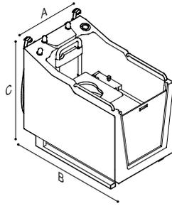
**800\_SHOWER CUBICLE WITH CONTROLS, INTEGRATED WITH TOILET, EQUIPPED WITH CHAIR WITH BACKREST AND SUPPORT HANDLES MADE OF STAINLESS STEEL WITH SATIN FINISH**
