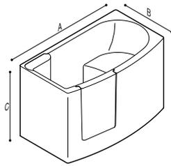
**655\_ BUILT-IN BATHTUB WITH DOOR OPENING INWARDS, EQUIPPED WITH DRAINAGE SYSTEM EMBEDDED IN THE FLOOR**
