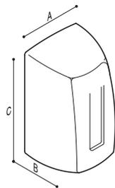
**STANDARD\_ FORCED AIR HAND DRYER, PHOTOCELL OPERATION, WALL INSTALLATION**
