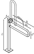
**PAINT\_ FOLDING SAFETY GRAB BAR ON FLOOR MOUNTED PEDESTAL**
