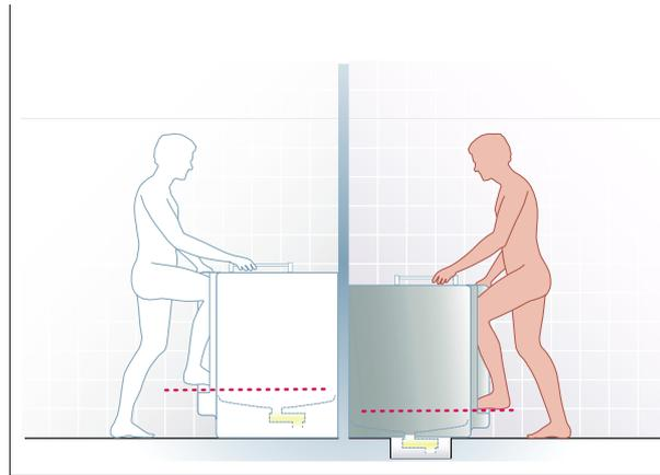
The bathtub with door - model 655 - offered by Ponte Giulio, has been designed to allow for it to be installed in two ways: either normally like any other one on the market, or with a built-in drain. The latter form of installation offers the opportunity to reduce the height of the step by 8 centimetres with respect to the floor, thus making it easier to access.
