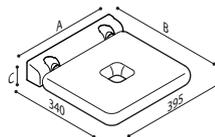
Material Polyurethane, Aluminium, Stainless steel, ABS
