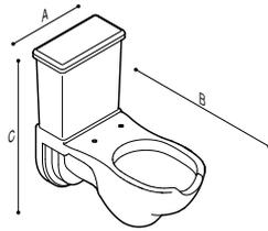
**ROSSARI\_ WALL-MOUNTED MONOBLOC TOILET, WITH FRONT OPENING, DUAL MODEL\_** If the pneumatic control with free position is used, request the items: H52HES01, H52HLS04 and choose the buttons on pages 144/146. For flush on the tank, request the items: H52HES05 and H52HLS04
