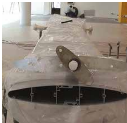
▲ Screw channels. In the front view of this CS Airfoil® AF380 blade the incorporated screw channels are clearly visible. The channels are part of the extrusion of the blade and run through its entire length. This allows for onsite cutting of the blade to any desired length and immediate fastening onto any fixing plate or bracket, saving time and effort during the installation process.
