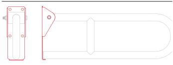
"Extended" plate Stainless steel with satin finish Stainless steel - AISI 304 [LxH] 82x220 mm.
