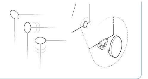
The mirror clip - F41JKS01 - is designed to secure mirrors with a thickness between 3 and 6 millimetres. It consists of three elements: a "delrin" disc, to keep the mirror about 3 mm away from the wall; an aluminium disc, to anchor the mirror to the wall using screws, a cover disc, used to block the mirror, made of AISI 304 stainless steel.
