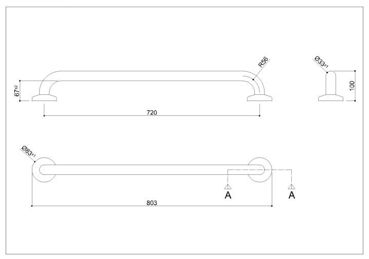
Straight grab bar made of seamless zinc-plated steel pipe, coated with antimicrobial, biocompatible and warm-to-the-touch vinyl
