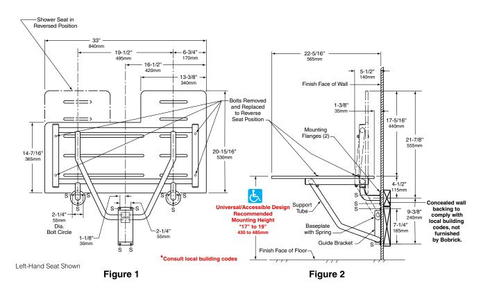
**Installation to Wall.** Secure unit to wall at points indicated by an *S*, with the two Mounting Flanges located at top and the Baseplate and Guide Bracket below. The bottom of the Support Tube must be positioned within the Baseplate and Guide Bracket before they are secured to wall. \* Mounting height of shower seat must comply with local building codes.
